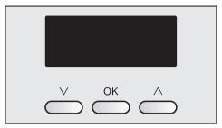
The display is operated using the ∨, **OK** and ∧ buttons. The value or option currently selected will appear highlighted.
